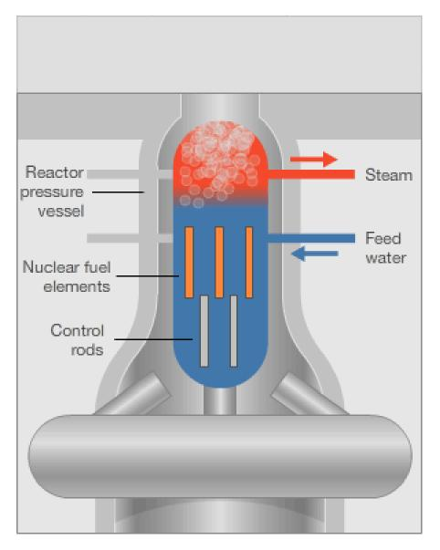
Each nuclear reactor heats water into steam; the steam turns turbines to generate electricity.
