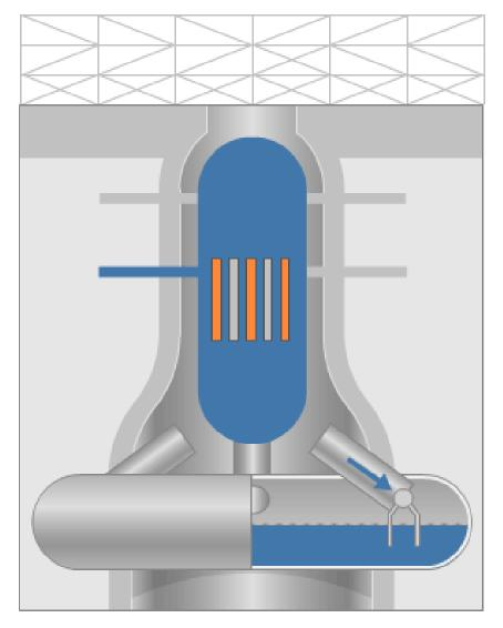
There are fears that the explosion at reactor 2 damaged its suppression chamber - a water-filled structure, which helps condense steam. If it has been breached, it may allow steam containing radioactive substances to escape continuously.
