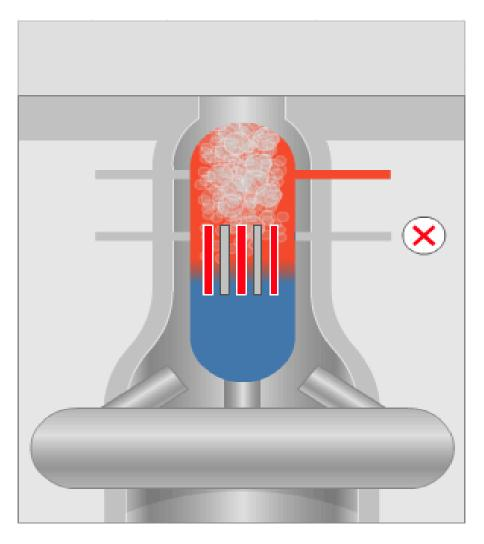
However, cooling systems failed because power supplies had been damaged by the tsunami.
