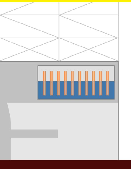
To bring the situation under control, power needs to be restored to the plant's damaged cooling system. Then, pumps can be used to bring the nuclear fuel back to safer temperatures.
