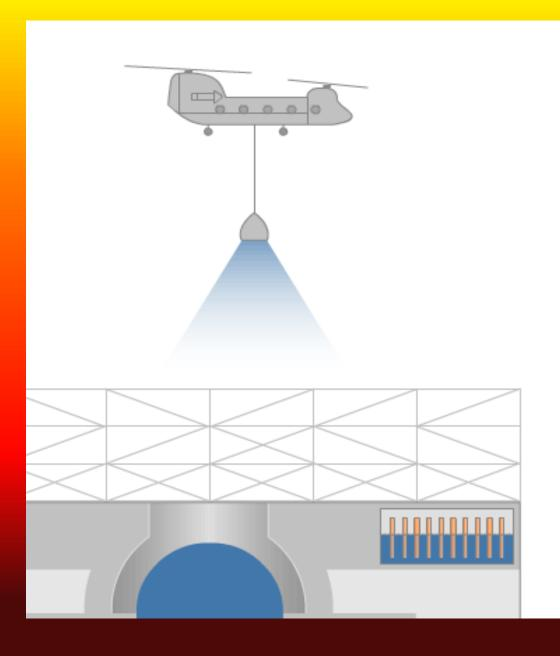
On 17 March, helicopters dropped water on reactor buildings 3 and 4, with the aim of replenishing water in storage ponds containing spent fuel rods.
