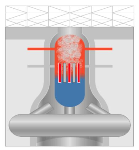
When engineers vented this gas and steam outside the pressure vessel, the hydrogen gas exploded, damaging the reactor buildings.
